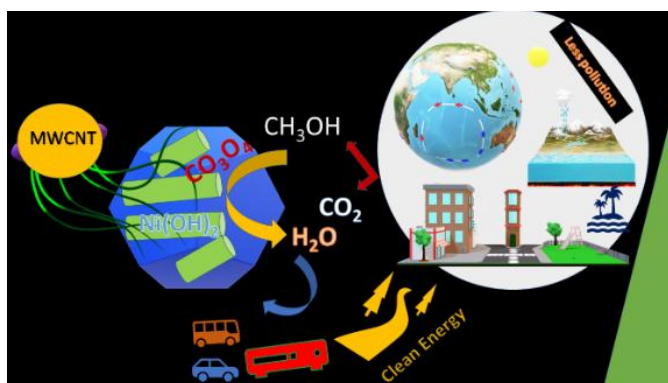
Scheme: ZIF derived Ni(OH) 2 -Co 3 O 4 -MWCNT electrocatalyst exhibiting good MOR activity
